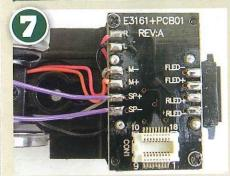
The decoder was removed to solder the speaker wires (each wire should be 120mm long) to the PCB.
