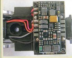
The compact size of the decoder is used to good effect by fitting it transversely.
