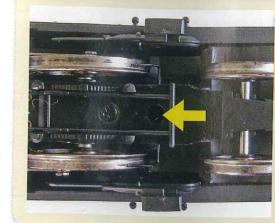
Remove this screw to allow the body to tilt forward. eleasing the forward retaining lug and allowing the body to be removed from
