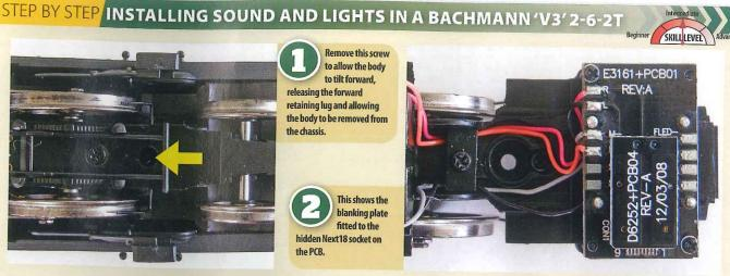
The latest generation LNER'V3' 2-6-2T features a new chassis design with a Next18 decoder socket and provision for installing a Zimo sugar cube speaker. This internal design makes the sound fitting process straightforward.
