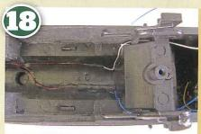
I fixed the wires in place with adhesive, checking that no fouling would occur on reassembly. This is particularly important near the rear driving wheels, but will be safe if passed though the mouldings as shown.
