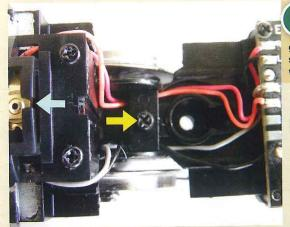
The blue arrow points to one of the speaker wiring guides, whilst the yellow shows the guide for multiple wires below the cab floor.
